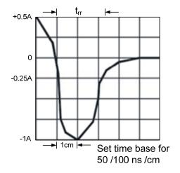
Notes: 1. Rise Time=7ns max. Input Impedance=1 magohm. 22pF 2. Rise time=10ns max. Source Impedance=50 ohms
